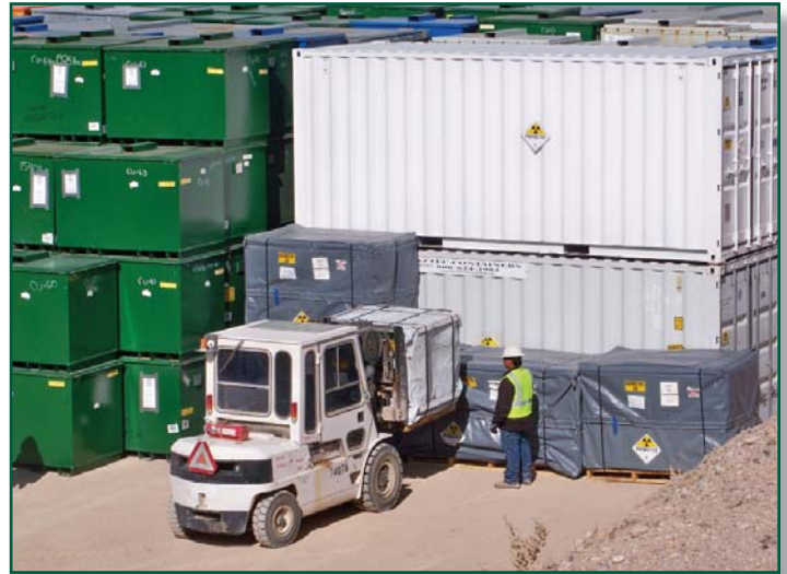
Waste packages are positioned in a disposal cell at the NNSS Area 5 Radioactive Waste Management Site
